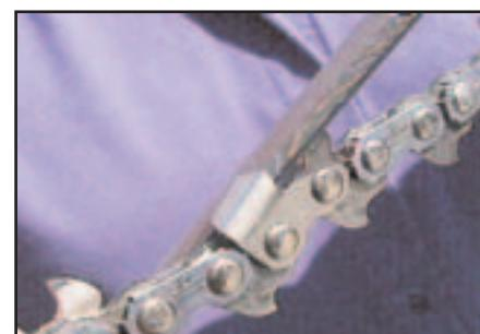
The "v" to the point is set with the bevel line at the edge of the larger flat file surface. Not the center line of the file's side bevel.
