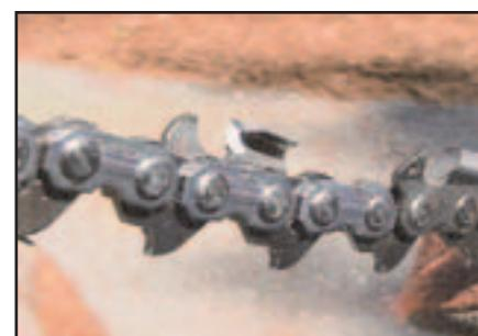
Square ground saw chain has a *channeled* cutting surface. This grind supports the point with a "v" and works more like a caving *v-tool* than a *gouge* action of a round filed saw chain.
