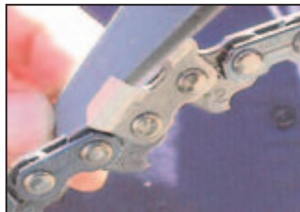
The angles of the file match the corner and the top plate chisel angle perfectly to form the channel.
